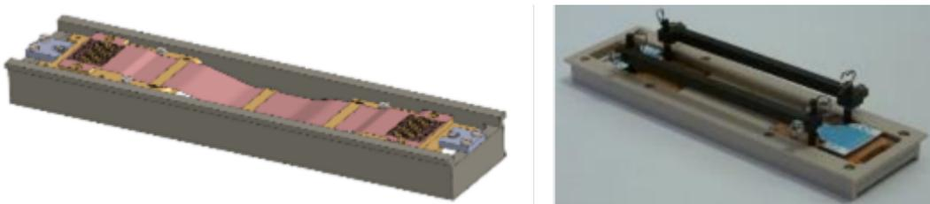
**Figure 13 : Support for the harness in the brazing machine. At right, in black, the top part of the handling tool is laid.**
