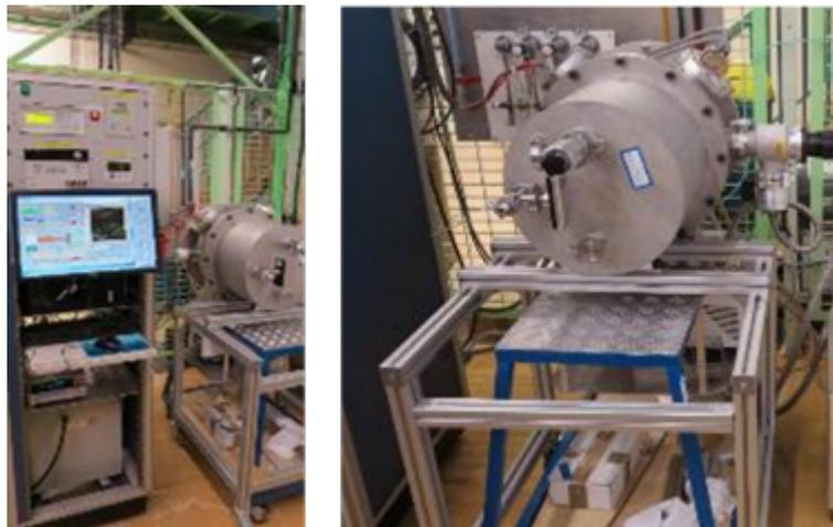
*Figure 18 : Cryo-cooler for the 4-wires measurement of the electrical resistance of the 37 tracks of an harness, according to the temperature.*
