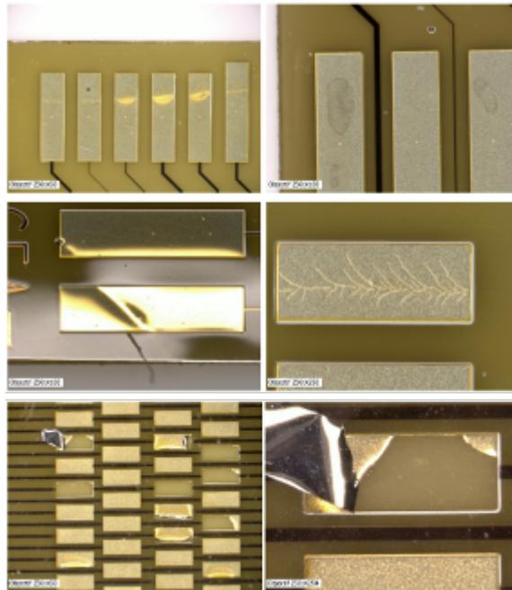
**Figure 7 : Delamination on connector's pads**
