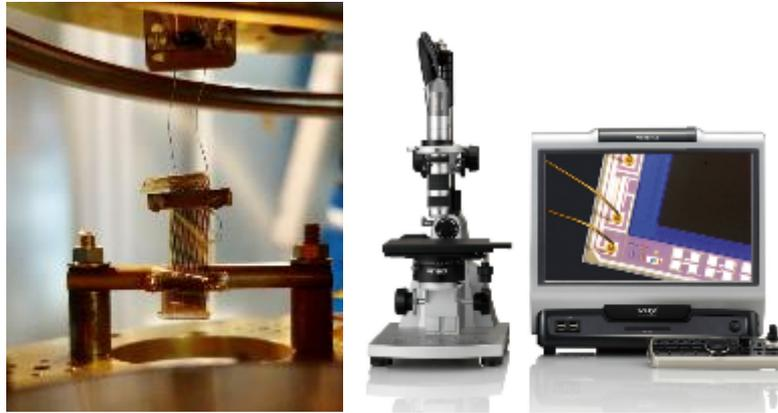
*Figure 17 : Left : test bench for the thermal conduction measurement. Right : advanced digital microscope for detailed visual inspection.*
