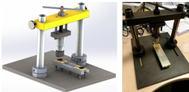
*Figure 10 : Heating press.*
