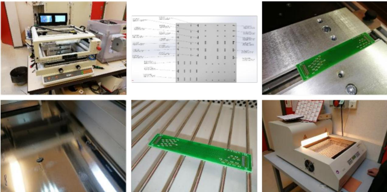
**Figure 12 : From left to right and top to bottom : brazing machine, stencil, dummy harness in FR4 PCB, spread of solder on stencil, passing in the oven, oven.**
