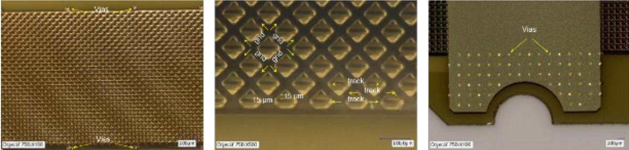
**Figure 5 :** At top : photograph of the harness. At bottom, left : zoom on the tracks and grids zone ; the shielding grids are closed by vias. Middle : further zoom where 15  $\mu\text{m}/15\mu\text{m}$  tracks appear between the two shielding grids. Right : zoom on a top thermal contact, with vias connecting it to the two shielding planes.
