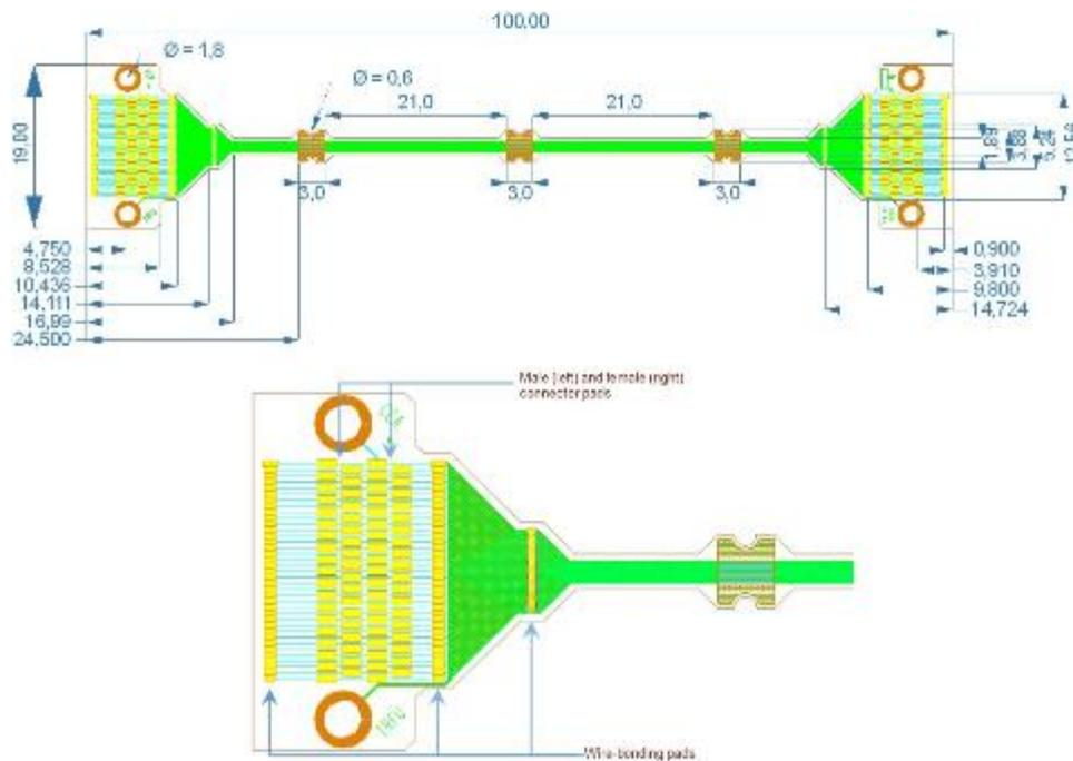
Figure 4 : Dimensions and interconnection.
