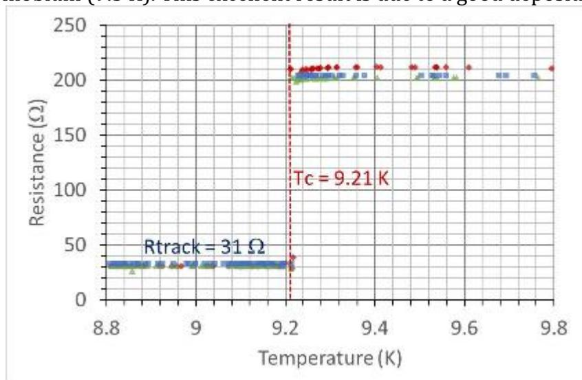
**Figure 6 :** Electrical resistance of three tracks (blue, red, green) versus temperature : transition around 9.2 K.
