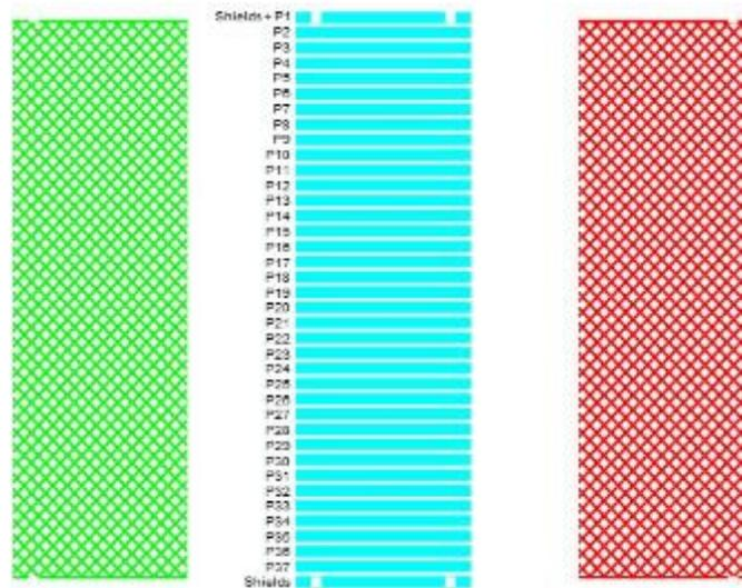
**Figure 2 : Section of the design of the top shielding layer (left), the signal layer (middle), and the bottom shielding layer (right).**
