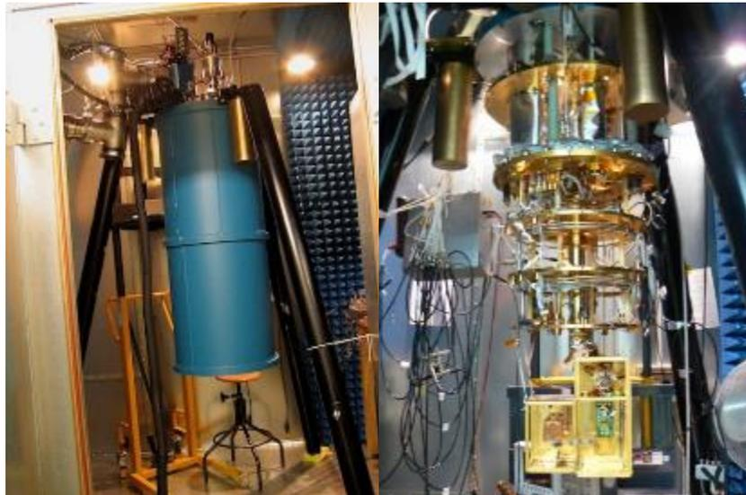
Figure 16 : Cryo-cooler for the measurement of the critical temperature of set of tracks.
