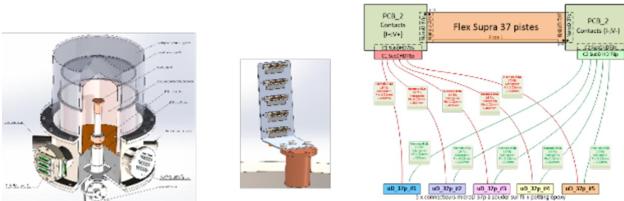
Figure 15 : Cryo-generator for the cycling of the harnesses. Cabling for the 4-wires measurement of the electrical resistance of the 37 tracks of an harness.
