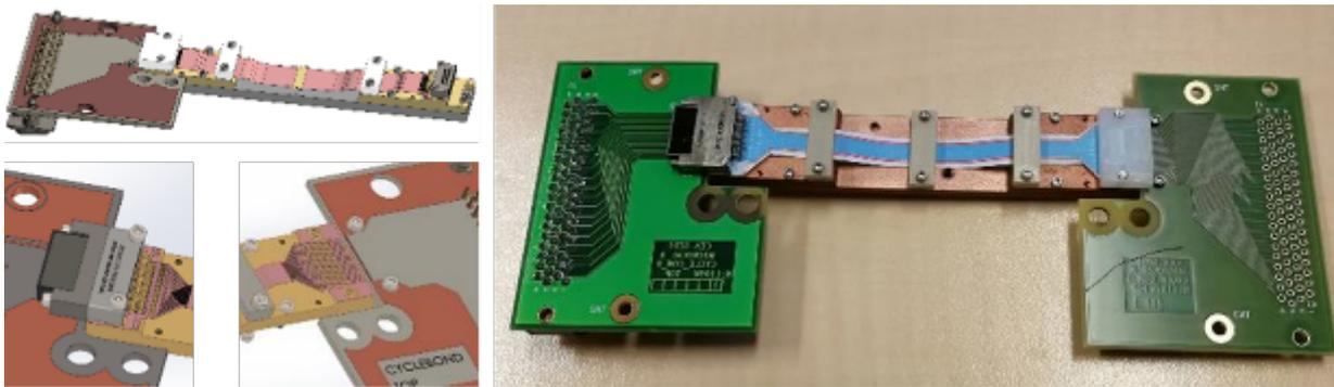
Figure 14 : Interconnection of the harness : connector configuration (left) and bonding configuration (right).
