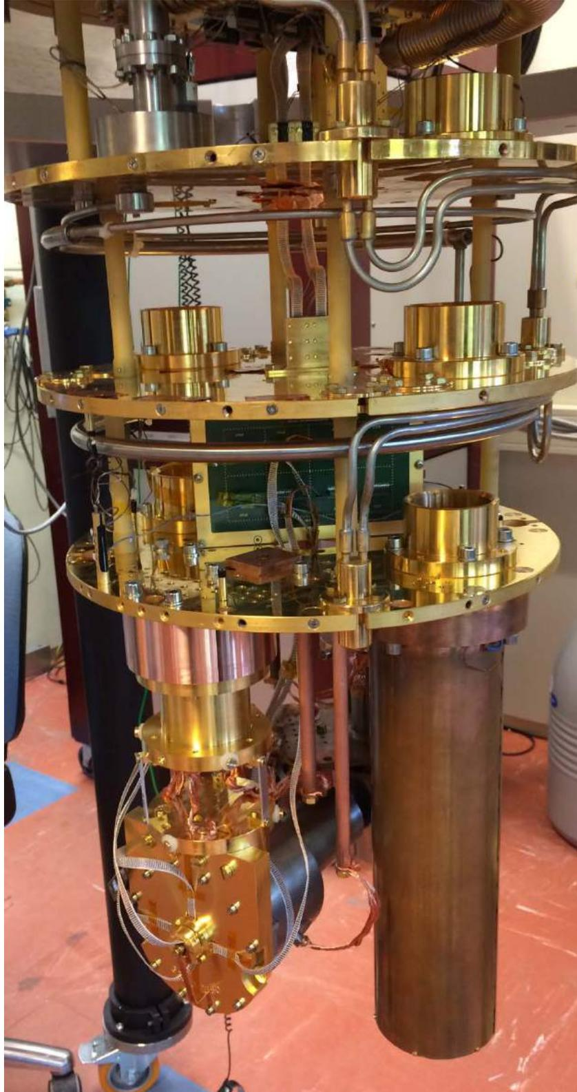
**Figure 22.** 40 pixel experiment location in SRON Utrecht LC-cooler, during Run 60.
