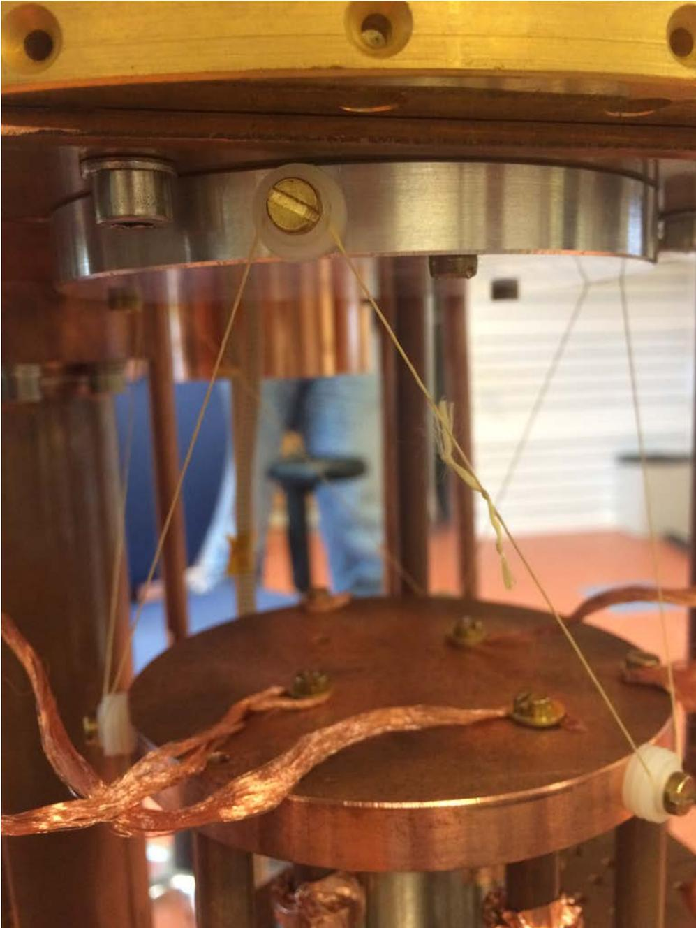
**Figure 13. Kevlar suspension, with copper thermalization straps to the 50mK plate.**
