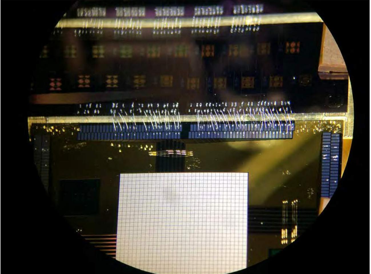
**Figure 15. GSFC LA1 mounted on 40 pixel FDM - A setup and connected with Al-wire bonds to the transformer chip. In Run 71 the array was rotated and Quadrant 1 connected instead of 3.**
