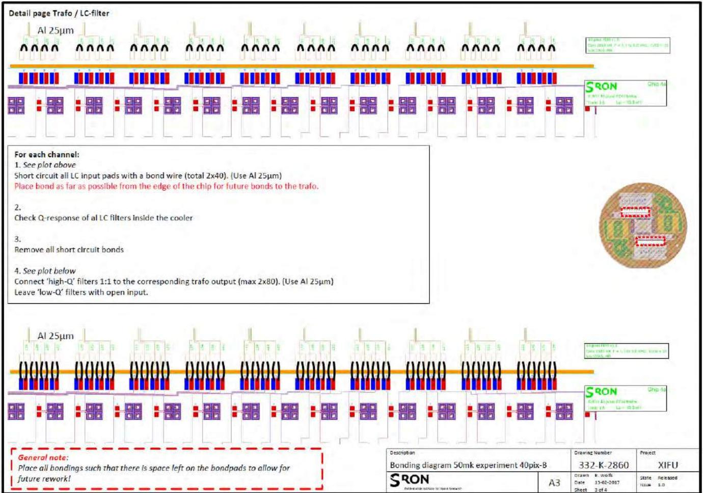
**Figure 4. Trafo - LC filter wirebond scheme, now 36/40 LC-filter have been connected to the transformer chip.**
