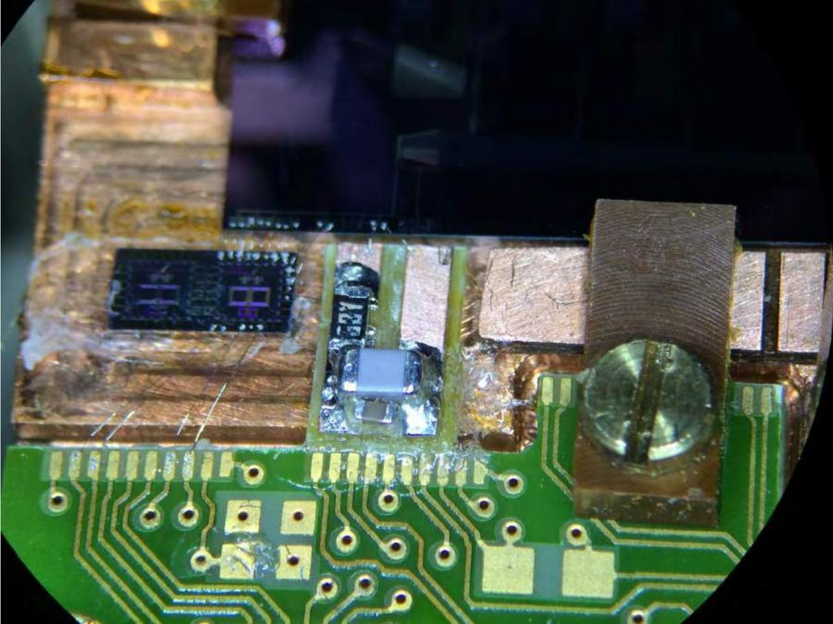
**Figure 7. Snubber / lowpass RC-filter circuit in parallel with Input SQUID.**
