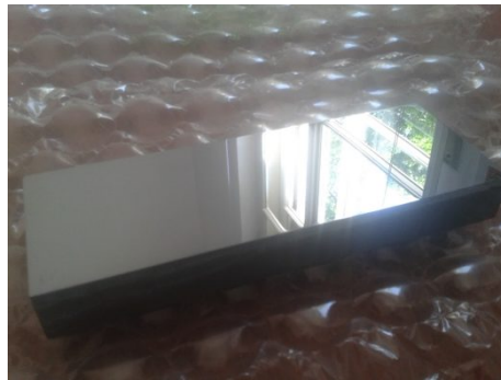
Figure 6: the beam expander crystal for the 4.51 keV setup, monocrystalline silicon, with the proper asymmetric cut at 44.59 deg from the (220) planes. The surface has been polished to remove the lattice damage introduced by the cut. The crystal dimensions are 170 mm x 60 mm x 20 mm
