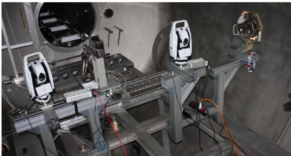
Figure 4. Integration set-up in the vacuum chamber of Panter X-ray facility
