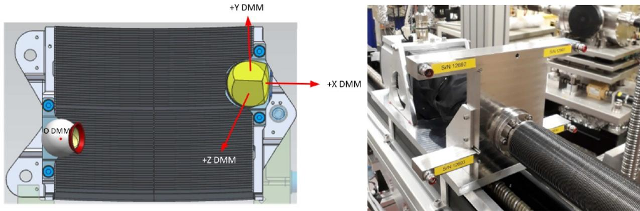
Figure 3. Optical fiducials positioned on the MM (left) and XPBF 2.0 detector stage (right)
