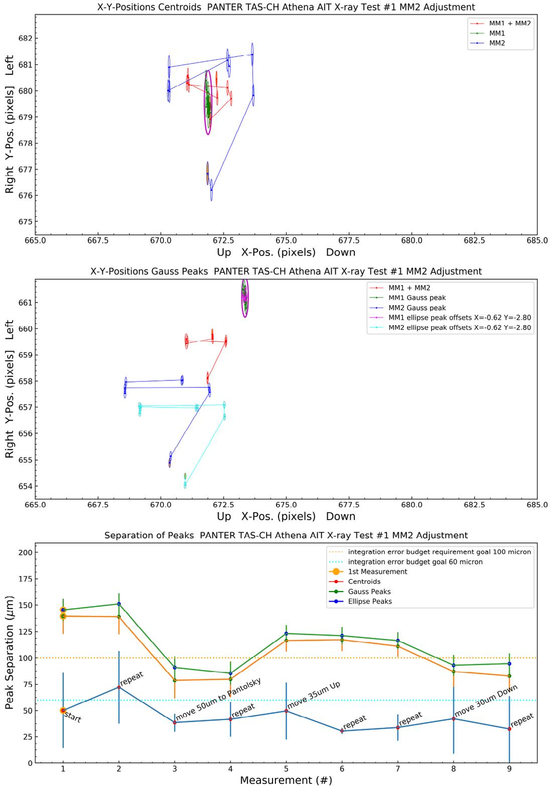
Figure 6. MM2 alignment under X-ray
