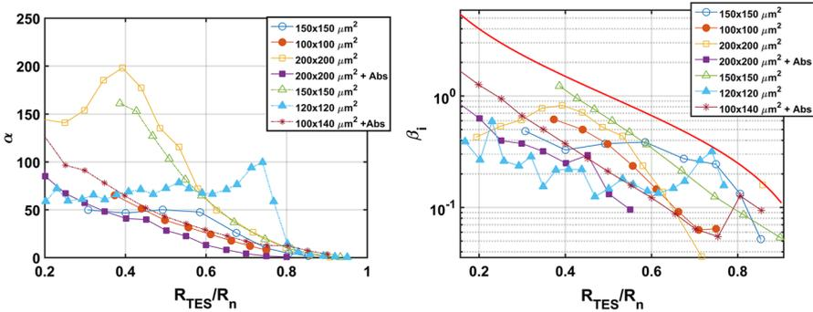
**Fig. 3**  $\alpha$  (left) and  $\beta$  (right) at 50 mK along the superconducting transition. Legends indicate TES bilayer dimension. Continuous line in  $\beta$  plot indicates weak link and phase slip regime separation [10]. The four upper TESs in the legend have banks, while the other three do not (Color figure online)
