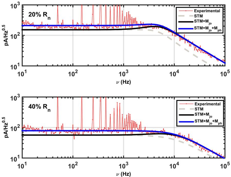
**Fig. 4** Two noise spectra of a representative TES (200  $\mu\text{m}$  side with absorber in Figs. 3), measured at  $T_{\text{bath}} = 50$  mK and at biases of 20 and 40%  $R_n$ , respectively. The solid lines display calculated noise using the experimental TES parameters and the simplest thermal model (STM) [1], as described in the text (Color figure online)
