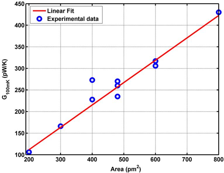
**Fig. 2** Thermal conductance scaled at 100 mK as a function of the radiative area, i.e., TES perimeter times membrane thickness (Color figure online)
