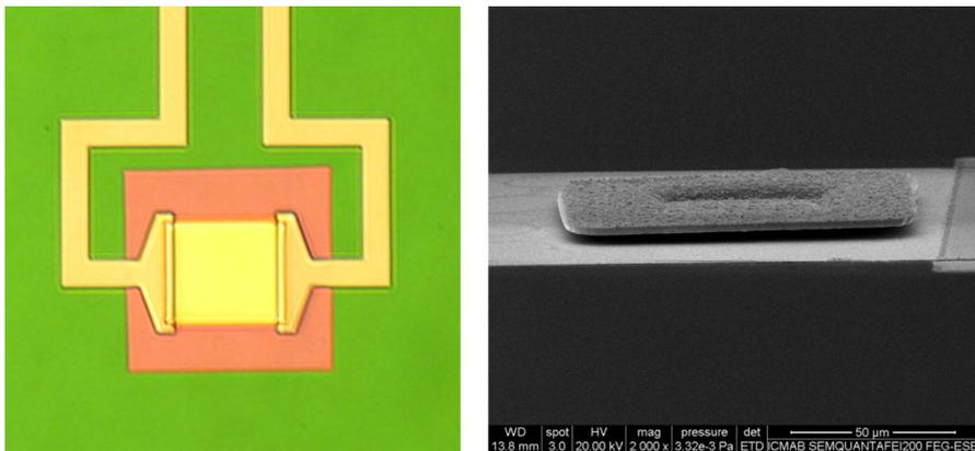
**Fig. 1** Optical photograph of a bare TES of dimensions  $120 \mu\text{m} \times 120 \mu\text{m}$  on a  $250 \mu\text{m} \times 250 \mu\text{m}$  membrane (left) and SEM micrograph of a mushroom-shaped Bi absorber on a TES (right) (Color figure online)
