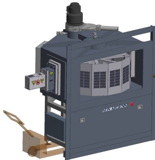
Figure 3. Schematics of the drum sputter coating system with the loading door removed, showing the carousel that moves carriers with SPO plates past three magnetrons. The chamber is about 2 m high, with a diameter of about 1.8 m and it can coat up to 100.000 plates per year.
