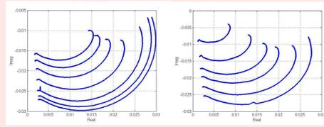
Complex impedance of a TES with T<sub>c</sub>=157mK, recorded at 138mK and 140mK, between 1kHz and 100kHz
