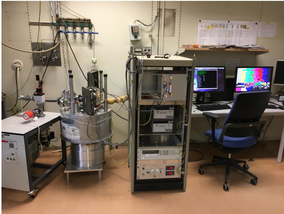
Fig 4.5: Complete FDM warm electronic system for the AHEAD2020 TES spectrometer project.
