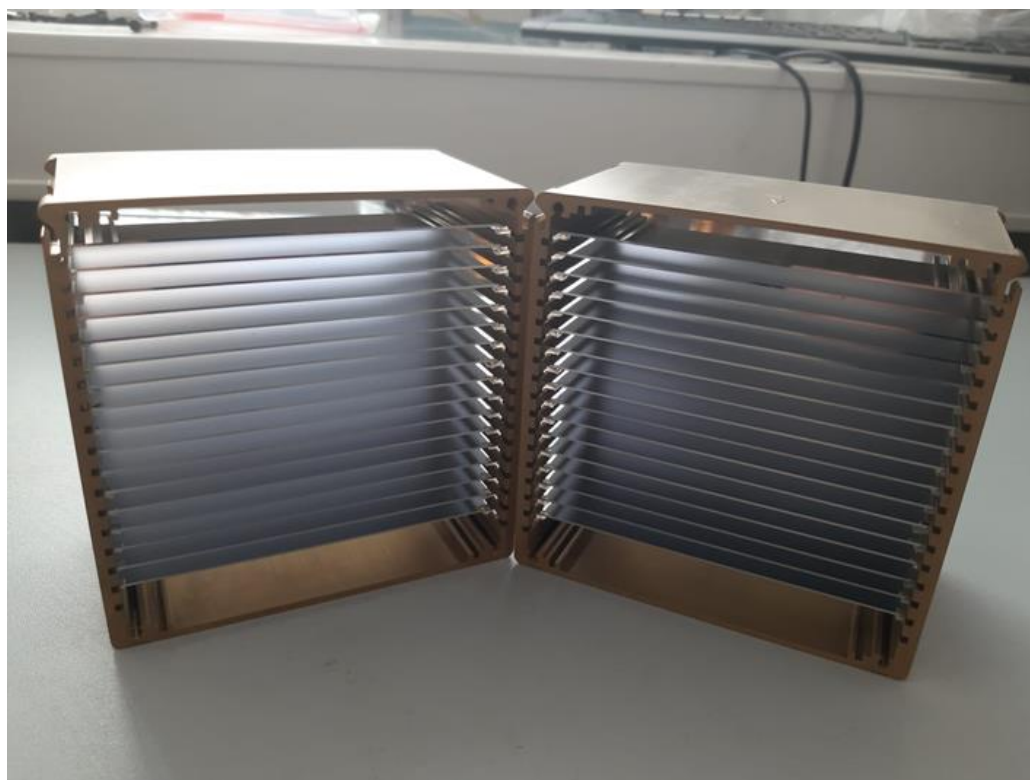
Figure 9 The double LE test module to experimentally compare different reflective layers with 4 x 17 Si wafers 0,625 mm thick, aperture 85 x 65 mm and f 2 m. Collaborative effort of CTU in Prague, Rigaku Prague, and Aschaffenburg University
