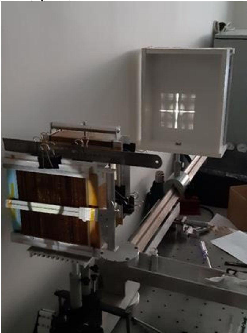
Figure 8 The LE test module with f=0.9\text{m} during testing in visible light.
