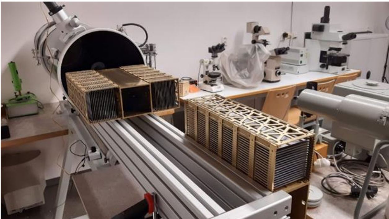
Figure 18 Large Kirkpatrick Baez Array during optical tests at the Prague CTU laboratory.
