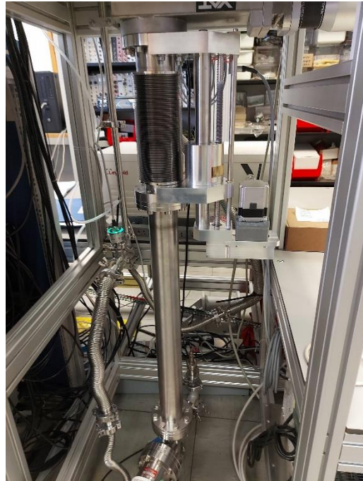
Figure 4: Extension added to the source section to try to make the source to optic distance equal to the optic to detector distance.
