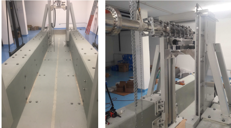
Figure 13: The detector tower. Left: holes to anchor the tower are prepared at f = 12 - 10 - 8 m, for flexibility of the facility. Right: The tower with the bellow for the focus search.
