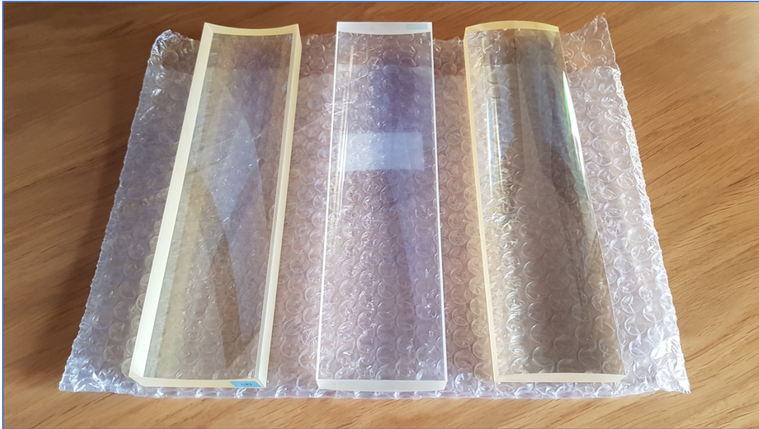
Fig. 25. The three lenses composing the cylindrical master
