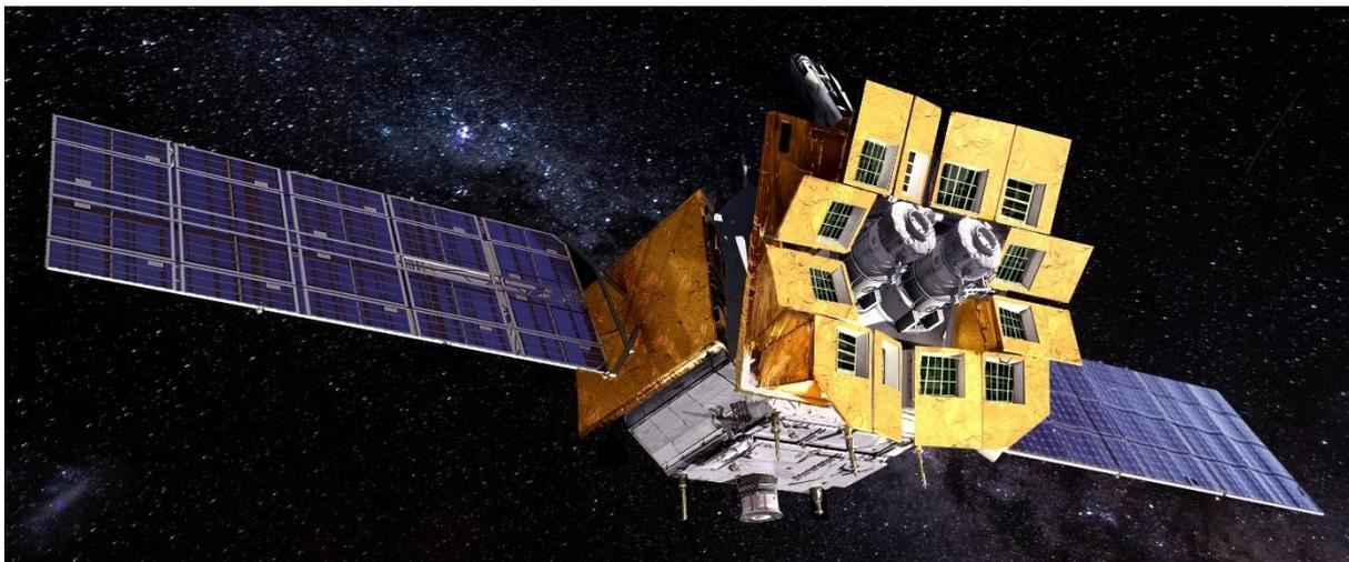
*Figure 2 Overview of the Einstein Probe observatory with the twelve WXT and two FXT telescopes onboard.*
