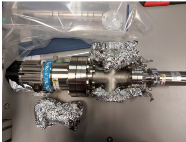
Figure 2: The source chamber. Turbo pump is on the left, gauge on the right, z-drive bellows above and electron gun at the bottom.
