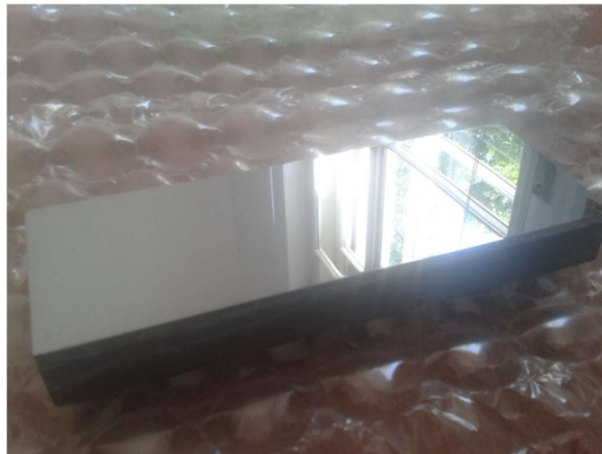
Fig. 14: the beam expanding crystal for the 4.51 keV setup, monocrystalline silicon, with the proper asymmetric cut at 44.7 deg from the (220) planes. The surface has been polished to remove the lattice damage introduced by the cut. The crystal dimensions are: 170 mm x 60 mm x 20 mm.
