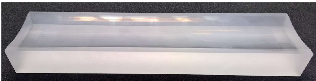
Fig. 16: one of the two paraboloidal mirrors procured from Carl Zeiss SMT GmbH, after the preliminary grinding. The mirror was subsequently lapped to partially smooth the periodic pattern left after grinding.
