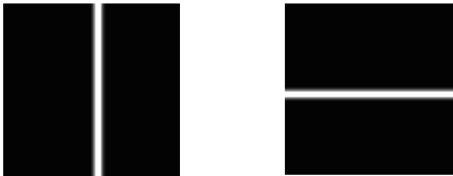
Figure 4: Ray-tracing simulation of 1D LE optics for sub-module A (left) and sub-module B (right) for source-detector distance of 7 m for ideal mirrors, ideal position.
