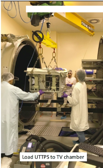
Figure 8: UTTPS Installation in TVT and end of test verification QM TVT Temperature Profile - part 2
