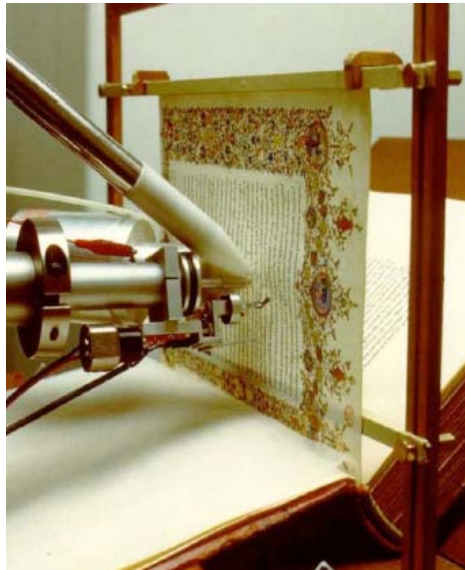
Fig. 5.1.3.1: example of PIXE analysis of an ancient manuscript (LABEC)
