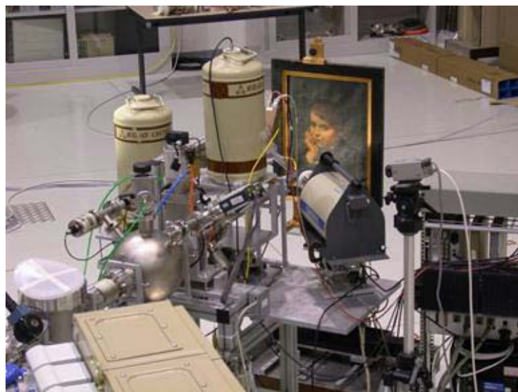
Fig . 5.3.1.1 a painting under examination at a PIXE facility (credit INFN, LABEC laboratory)
