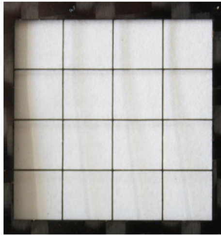
Fig. 11 A mini-mesh 2 \times 2 cm with 5 mm pitch and 0.15 mm wire width manufactured at O. R. Lasertechnologies by cutting a commercial 0.25 mm thick pre-impregnated C-fibre sheet with a fibre laser
