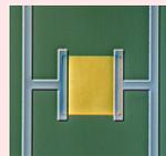
Optical and SEM micrographs of a Mo/Au TES
